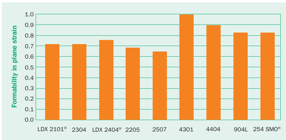
Fig 13. Formability ranking of some duplex and austenitic grades in relation to grade 4301.
